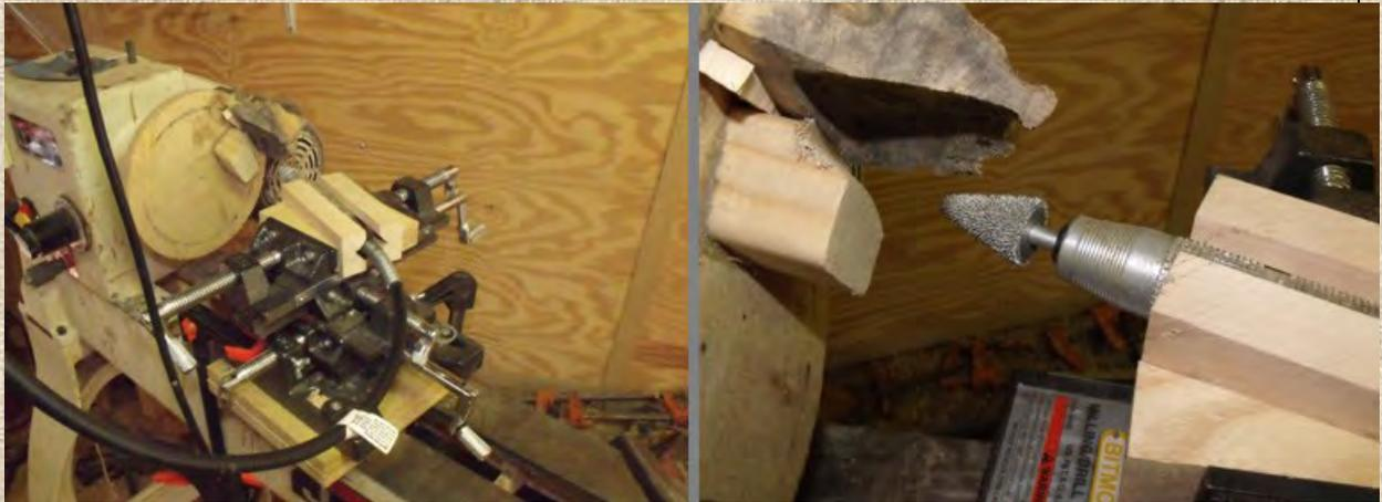
Although I think this could have been done without the milling vise and power carver, cutting this with only the lathe and cutting tools would require that you cut very blindly into a spinning piece of fragile wood.
