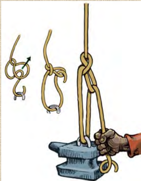
Trucker's hitch – very useful when tightening a line over a load and easily pulls loose after you're finished. If you tie it correctly.
