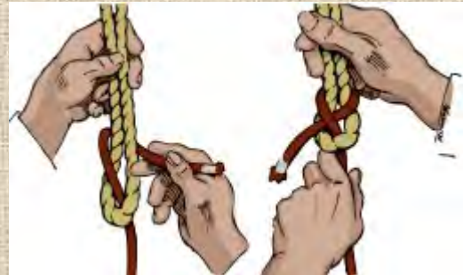
Sheet bend – Excellent for attaching two lines together, but works best when connecting lines of differing diameters.
