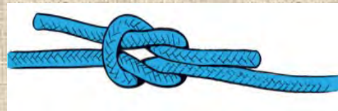
Square knot – the first knot I ever learned to tie...right over left and under; left over right and under.
