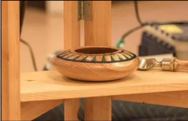
**Nick taught us how he lays out his designs and geometric patterns using the index function on his lathe or by utilizing round compasses downloaded from the internet. He went on to grind recesses in his bowl, making them ready to be filled with crushed stone**
